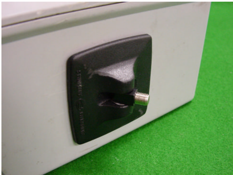
Glass Mount DAB Band 3 / L Band Antenna : Screw Mount on Box
